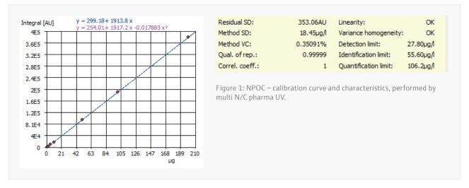
An outstanding linearity could be demonstrated throughout the whole calibration range from 0.1 to 20 mg/L for all three analyzer models of the multi N/C pharma series.
