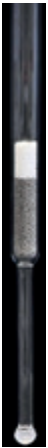
Figure 5: New filling of the combustion tube (high temperature mat, Pt-catalyst and Pt-grid on the bottom)
