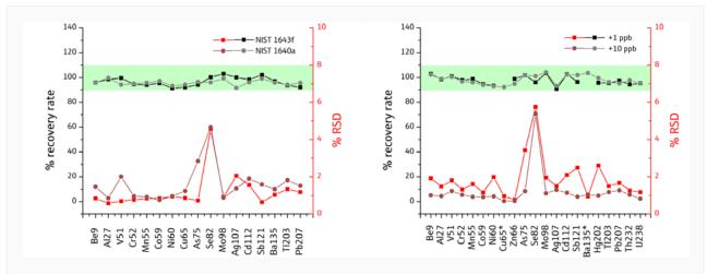
Figure 3: Recovery rate and precision of certified reference materials and lab-fortified blanks. All measurements are within the range specified. The spike concentration of +1 ppb was <5 % of the sample concentration for Cu and Ba and was excluded.
