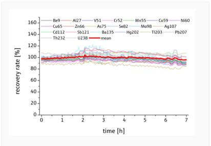
Figure 5: Recovery rate of the certified reference materials and LFMs as a function of time. Stable and accurate results were measured on all masses for 7 hours proving the robustness of instrument and method.
