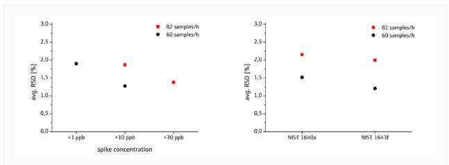
Figure 4: RSD of matrix spikes and certified reference materials measured with two different speeds. The outstanding sensitivity allows to measure 82 water samples per hour with competitive precision.
