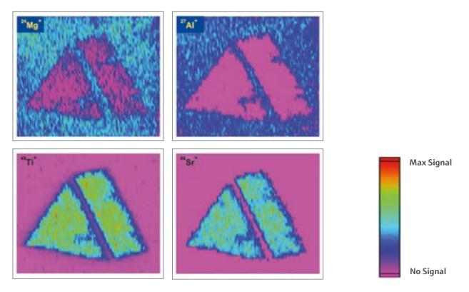
Figure 2. LA-ICP-MS elemental maps based on Mg, Al, Ti, and Sr signals obtained from the Analytik Jena ICP-MS combined with the J200 Tandem instrument.
