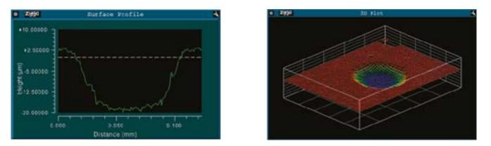
Figure 1. Laser ablation crater (60  $\mu$ m spot) displayed using a white-light interferometric microscope (Zygo). The crater is a result of 25 laser pulses from a 266 nm laser at 0.57  $\pm$  0.01 mJ
