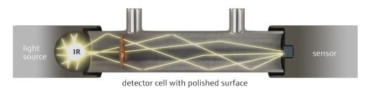
Fig. 1: Schematic structure of a conventional NDIR detector (image: Analytik Jena)
