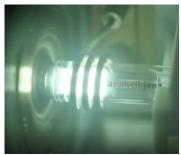
Figure 2: Hot plasma at 1.5 kW
