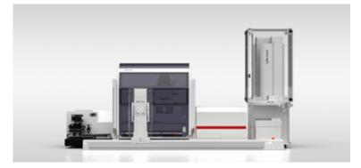
ELISA platform – 1400 mm CyBio Carry 1400 combined with CyBio FeliX automated liquid handler, CyBio QuadStack labware stacker (Analytik Jena), FLUOstar Omega-Reader (BMG Labtech) and EL406-Washer (Biotek)
