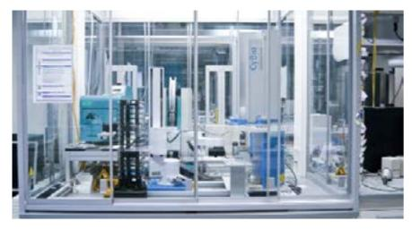
The Dilution System automates assayready plate preparation, reformatting and serial dilutions based on the TTP Labtech Mosquito® technology. A sophisticated data base management combined with a 4-axis laboratory robot, storage and a sealer, allows for high flexibility and increased walkaway time.
