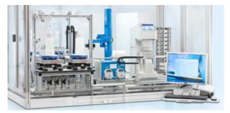
Designed for 24/7 operation, our elution system automates the purification of custom made DNA/RNA oligonucleotides on a production scale. The heart of the system is a multichannel-dispenser and vacuum-filtrationsystem that is complemented by our pipetting technology, a storage system and a 4-axis laboratory robot.
