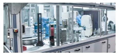
The Automated Plate Replicator is capable of producing large numbers of storage and screening plates and ensures sample integrity during transferring aliquots of compound from a library stock. It combines our liquid handling with REMP tube technology and handles the plate transport by two 6-axis robot systems.
