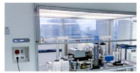
Setup in a level 3 laboratory, the Virus Screening System is primarily used to semi-automate the study of retroviruses, including HIV. Our pipetting and dispensing technology is supplemented by an integrated washer, different storage systems as well as a 4-axis laboratory robot.v
