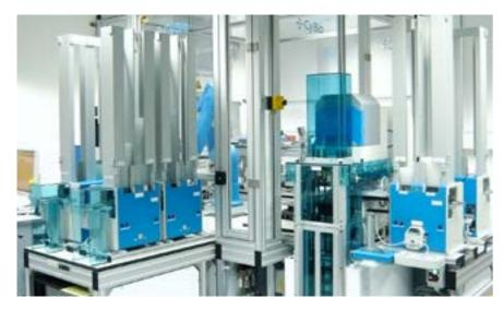
The CyBi®-Screen-machine is designed to allow flexible and reliable automation of antibody-based immunoassays. Based on a 6-axis robot system to handle the plate transport, the range of integrated instruments automates the processes completely.
