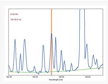
Figure 1: HR ICP optical emission spectrum of the B182.581 nm line in high-alloyed steel
