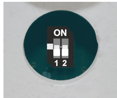
Modules positioned after gas sampling system: Dip switches 1 + 2 in lower position
