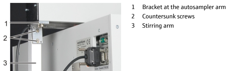
Fig. 27 Fitting the stirring arm to the autosampler
