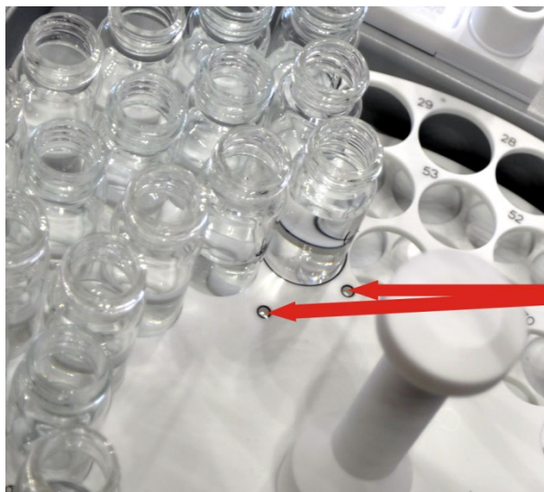
Fig. 53 Adjustment points on the sample tray
