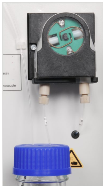
Fig. 9 Phosphoric acid pump
