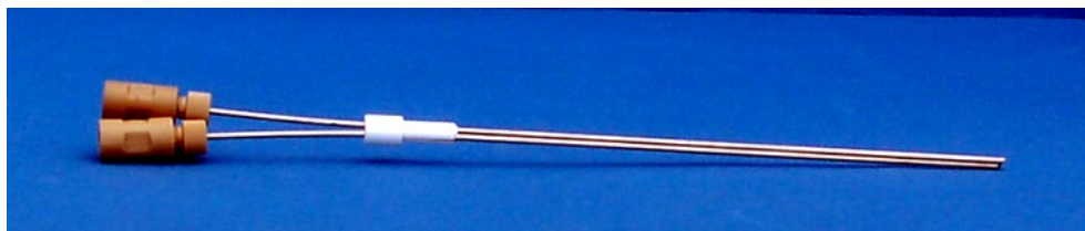
Fig. 22 Sleeve with 2 cannulas for NPOC measurements (non-parallel purging)
