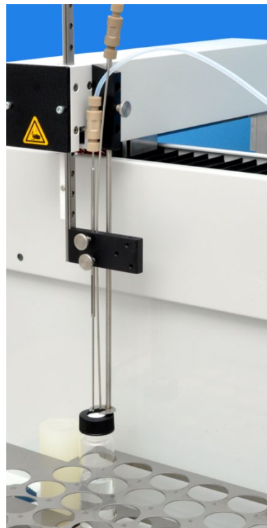
NPOC measurements with non-parallel purging: Insert both cannulas into the left position in the cannula holder
