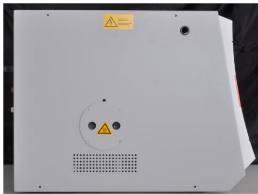
Left-hand side with dust trap contact guard
