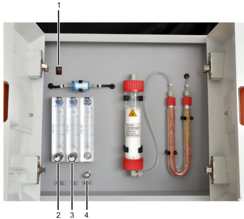
Figure 7 Control elements behind the front door of the multi EA 4000
