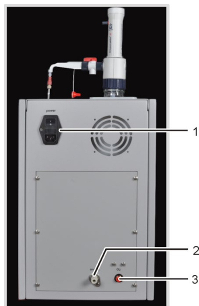
Figure 31 Connections at the manual TIC solids module
