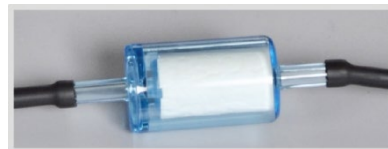
Figure 24 Dust filter before the changeover valve
