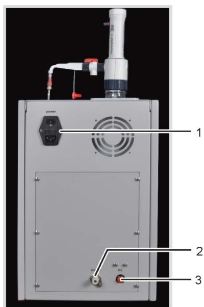
Fig. 29 Connections at the manual TIC solids module
