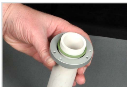
Fig. 31 Individual components for the connection between the TIC reactor and ceramic tube
