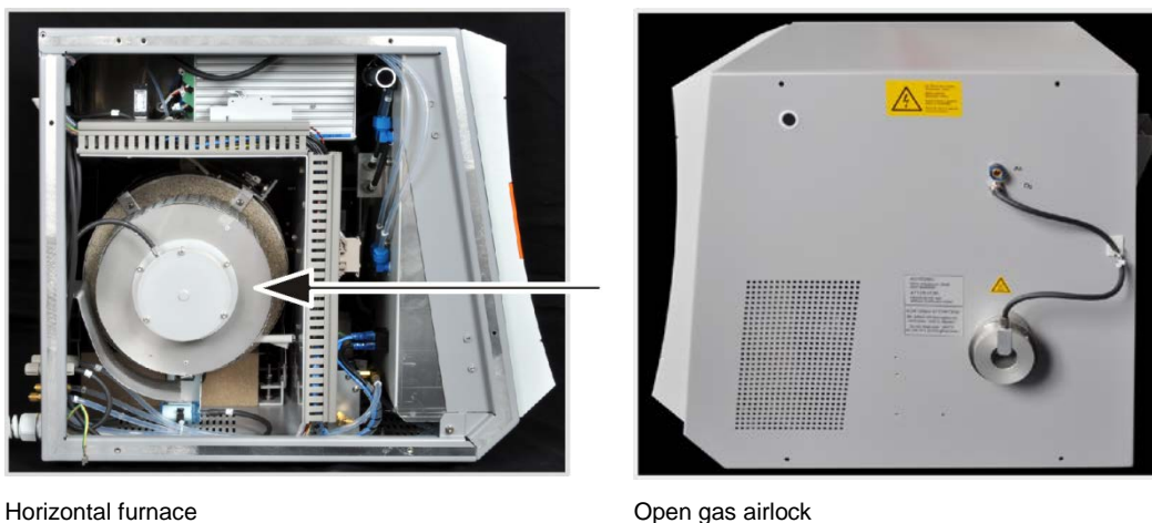
Fig. 1 Horizontal furnace of the basic device multi EA 4000
