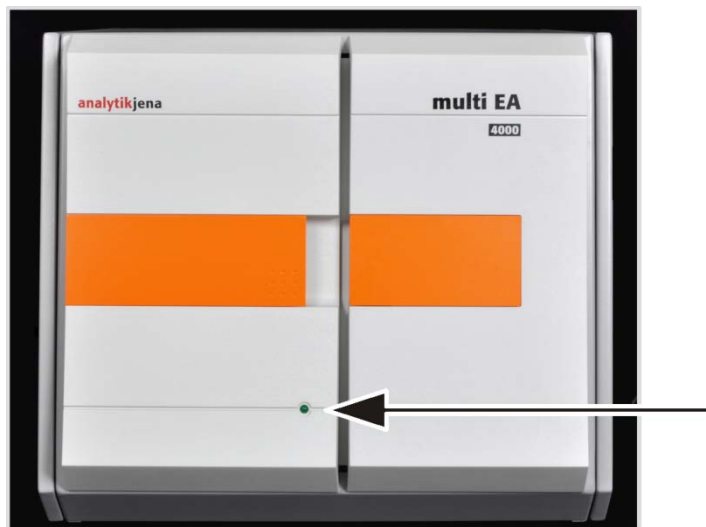
Fig. 5 Status indicators at the basic device multi EA 4000
