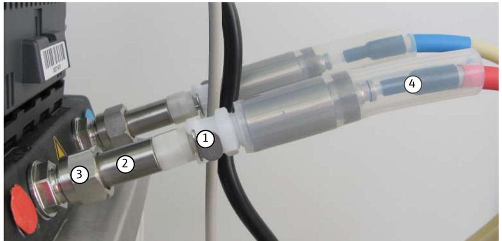
**Fig. 18 Thermostat - Raccords**
