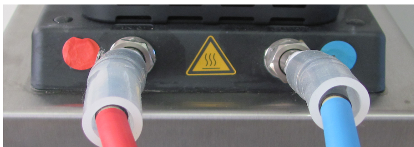
Figure 19 Thermostat – connections at the rear
