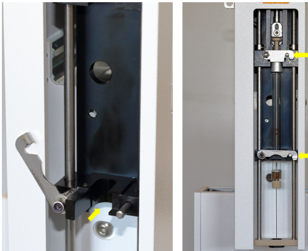
Figure 24 Syringe adapter and interlocking tabs
