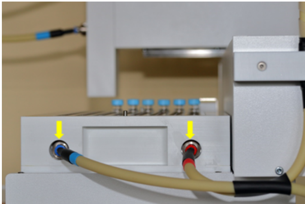
Figure 23 Connection to the temperature-controlled sample tray
