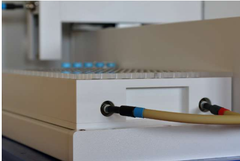
Figure 17 Temperature-controlled sample tray – connectors
