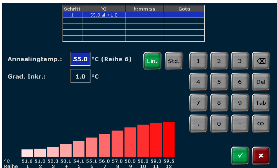
Abb. 22 Biometra TOne Linear Gradient Tool Bildschirm
