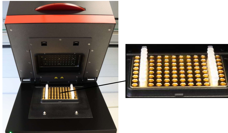
Figure 11 Positions of additional 8-well strips when measuring with few samples
