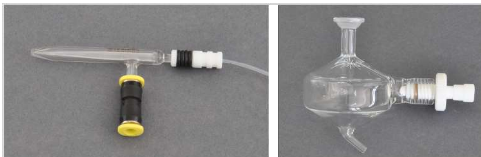
Figure 5 Concentric nebulizer and spray chamber
