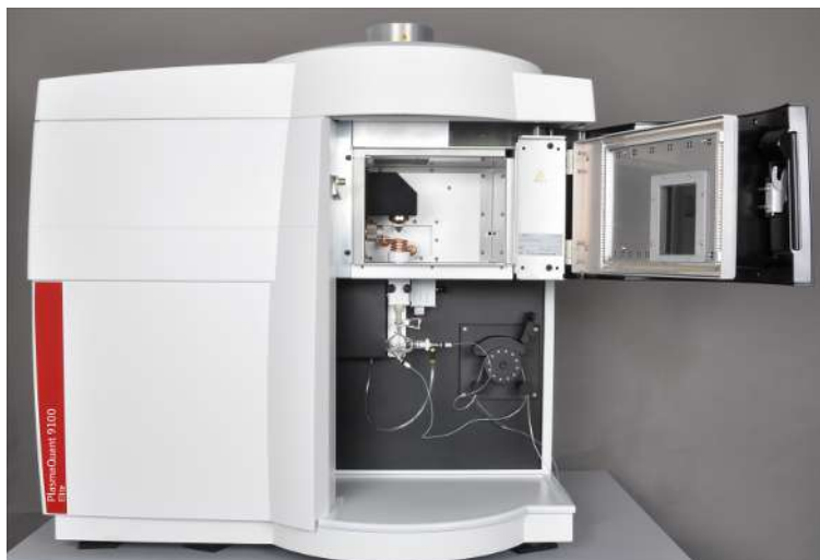
Figure 1 Emission spectrometer, with opened plasma compartment
