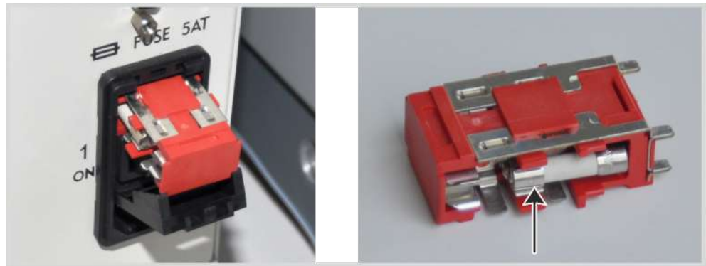
Figure 37 Replacing the fuses on the sampler
