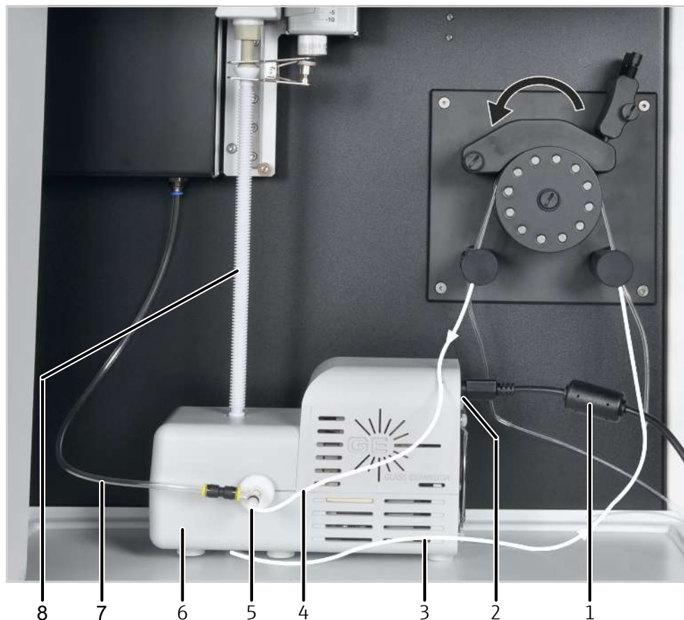
Figure 26 Installing the temperature-controlled spray chamber
