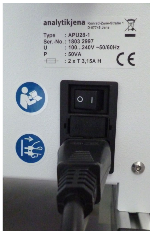
Figure 10 Main switch on the rear of the device
