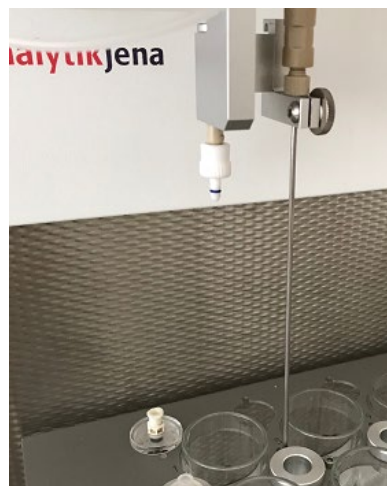
Figure 17 Dosing head not at the final depth
