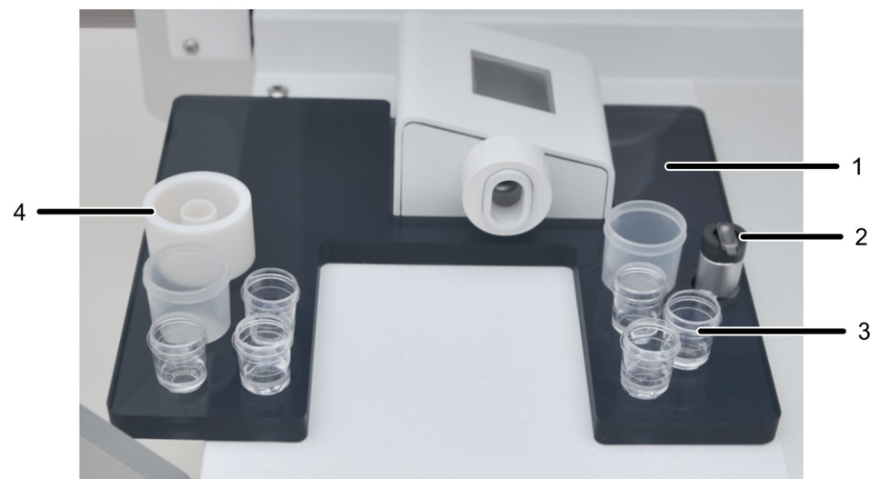
Figure 6 Sample holder for liquid dosing unit
