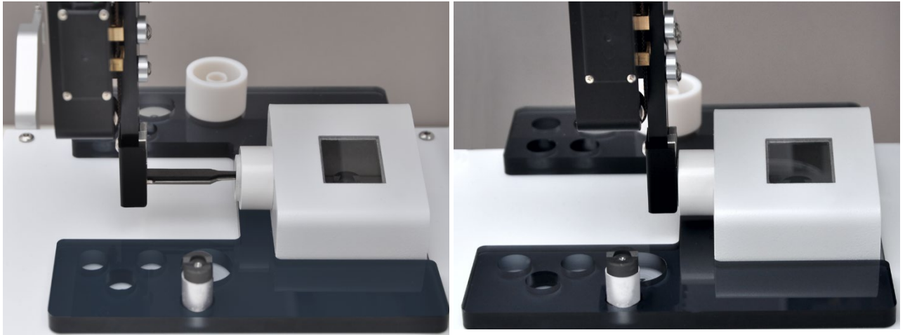
Figure 5 Scales with wind protection hood and sample port
