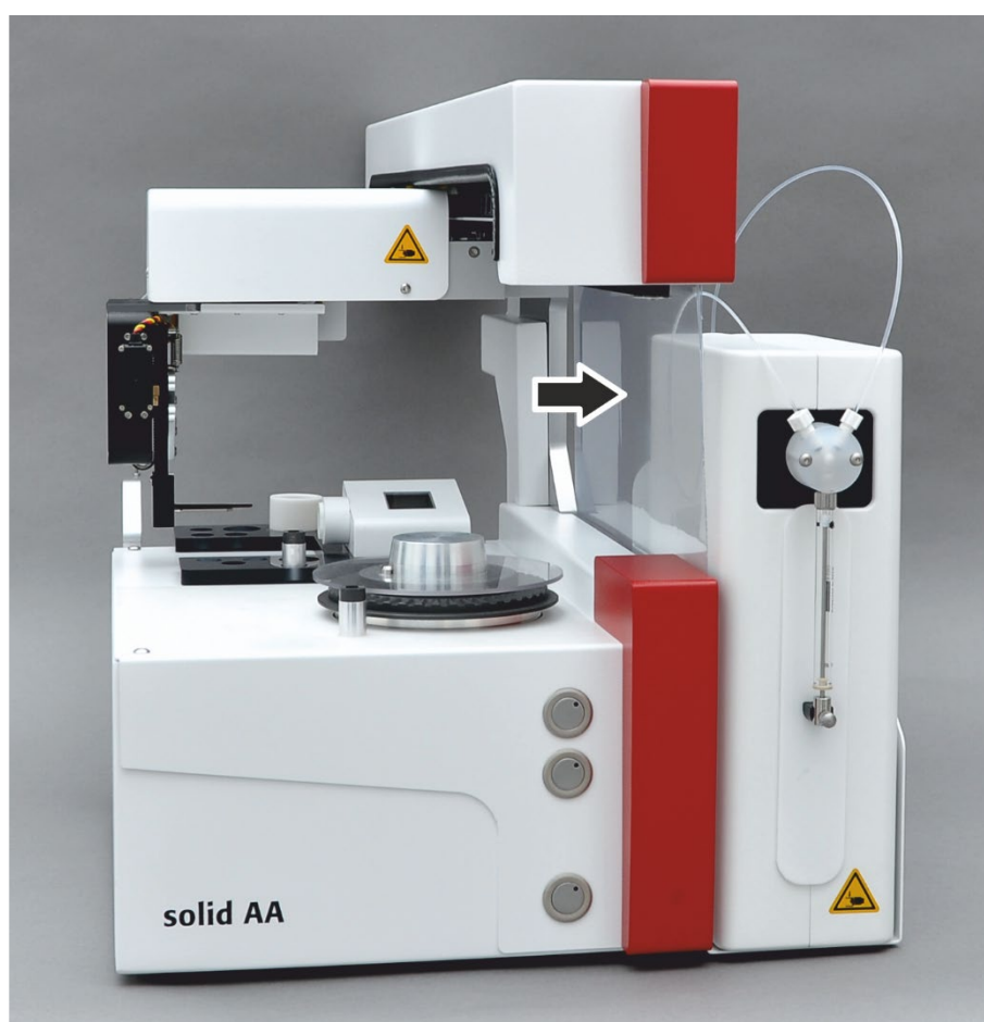
Figure 21 Protective film at the SSA 600 (arrow)
