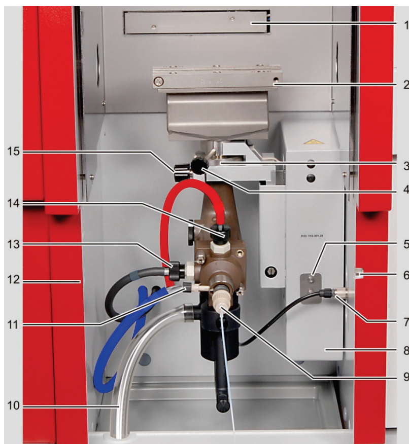
Fig. 39 Connections to the burner-nebulizer system in the sample chamber
