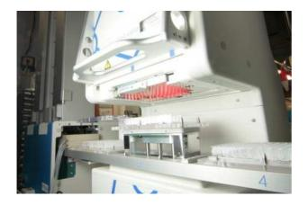
Figure 1: The CyBi®-Well vario Capillary Head with inserted 96 capillary magazine and 50 nl capillaries as well as a summary of the different capillary types.
