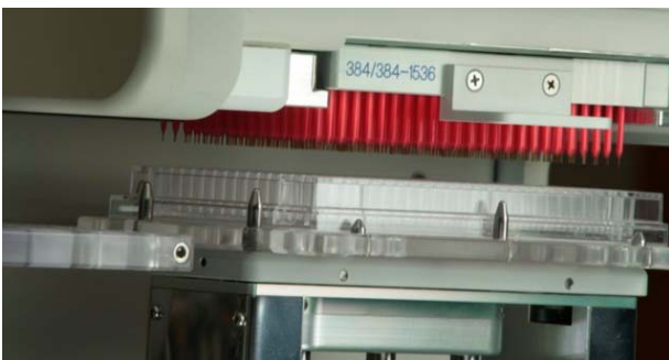
Figure 1: The CyBi®-Well vario Capillary Head with inserted 384 capillary magazine and 50 nl capillaries as well as a summary of the different capillary types.
