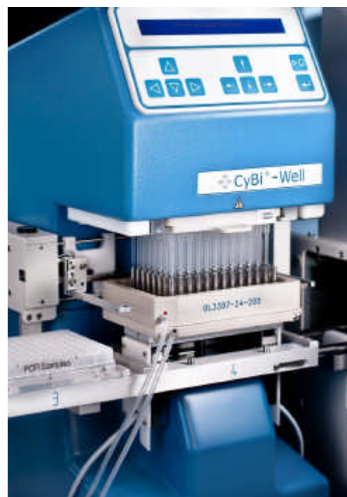
Figure 1: This figure shows the CyBi®-Well 96/250 µl equipped with an active deep well Tip Wash Station 96, which was used to optimize the tip washing after DNA sample transfer.
