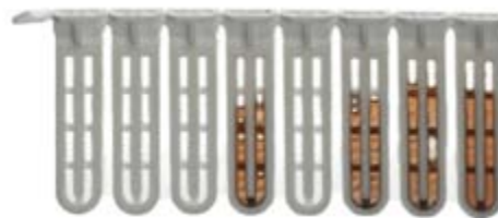
▲ Figure 1: One cartridge of micro dialyzers MD100 with 8 micro dialyzer units
