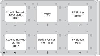
Figure 2: CyBio® FeliX deck layout for automated extraction using smart Blood DNA Midi prep (a96).
