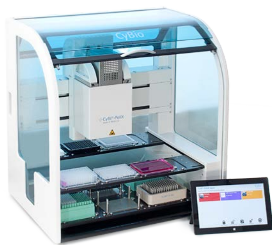
Figure 2. The CyBi®-FeliX possesses a small footprint with sufficient deck positions for reagents and labware consumables. Users may customize the instrument configuration to meet their specific needs.
