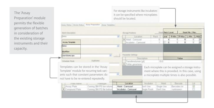
Batches are generated in the CyBio® Plate Tracking module, it being possible to specify different properties, such as type of microplate, barcode, lid etc., for each assay. The option to define workflow parameters permits the creation of flexible workflows; of course, both workflow and microplate
