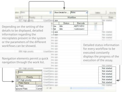
For every instrument, the microplates present in the instrument can be displayed. Therefore, it is possible to obtain an overview of which microplates are at which positions in the system at all times.
