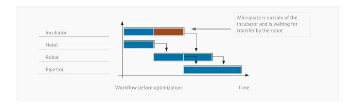
To this end, starting times for process steps are adapted such that no holding times occur between the individual steps, as far as possible. This makes it possible to achieve a higher throughput and the period of time that microplates are outside of a tempered environment can be shortened.
