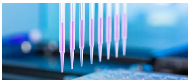
CyBio FeliX with Head R 96/60 µl and an 8-channel adapter using 50 µl tips
