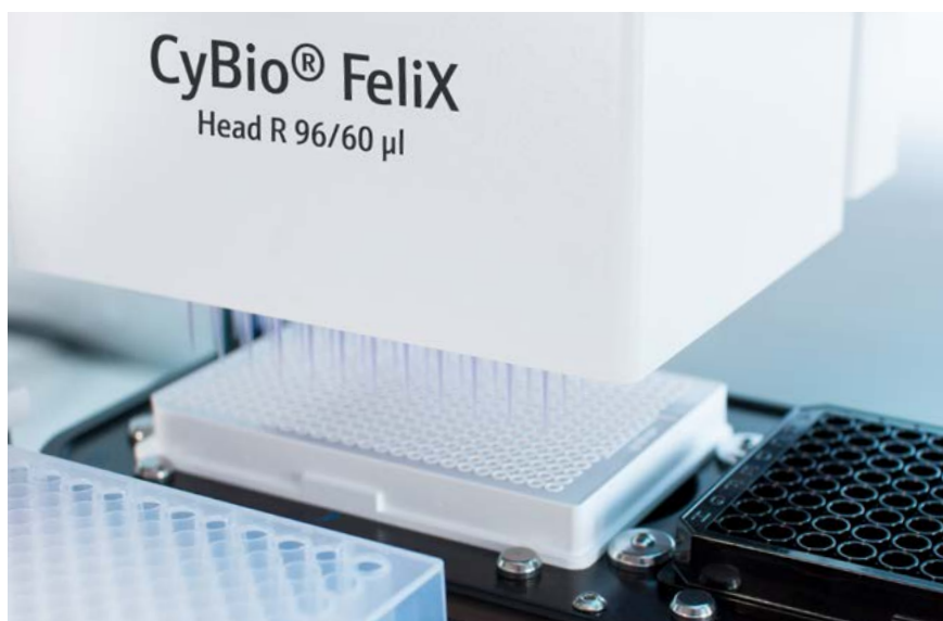
CyBio FeliX with Head R 96/60 \mu l and a CyBio RoboTipTray 96 with 60 \mu l tips
