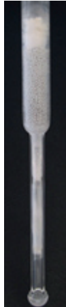
Figure 6: Combustion tube after 800 brine injections (salt deposits on the colder exit part of the tube)
