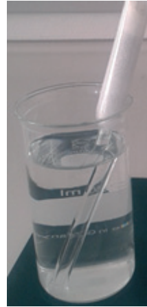
Figure 7: Re-dissolving the salt crystals by immersion into ultra-pure water
