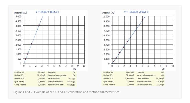
Within the method up to 3 calibration ranges can be linked to each parameter in order to cover an over-all working range of up to 3 magnitudes. Detection limits and limits of quantification are depending on the selected working range and can be derived from the method characteristics given above.
