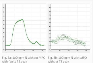
The analysis curves of the sulfur-free 100 ppm N standard prove the effectiveness of the MPO technique as a valuable tool to eliminate the interfering NO completely before analyzing the TS content.
