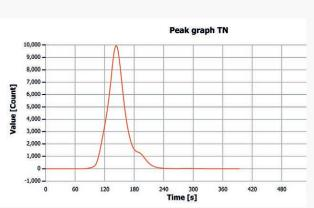
Figure 1 b: TN measuring curve for crude tall oil
