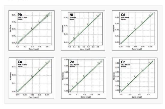
The measurements were performed using a novAA® 800 F for flame AAS, equipped with injection switch SFS 6.0 and an autosampler with automatic dilution function. The analysis was carried out using a 100 mm burner head for air/acetylene flame.
