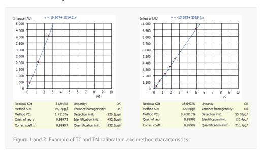
Within the method up to three calibration ranges can be linked to each parameter in order to cover an over-all working range of up to three magnitudes. With the NPOC/TN<sub>b</sub> method three NPOC and two TN<sub>b</sub> multi-point calibration ranges were linked as follows:
