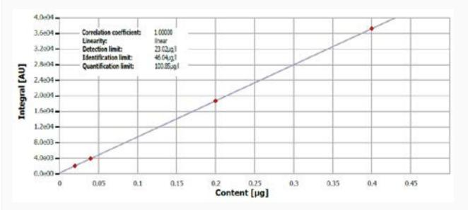
Figure 1: Examplary calibration for TN upper range, curve including statistics
